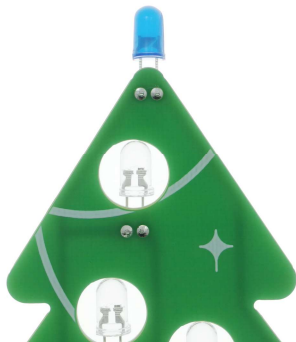
Fot. 4 Wlutowane diody LED
